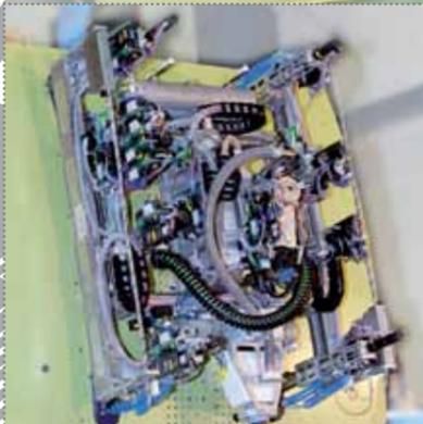
After drilling/riveting at the current area, the FDH walks one more step, by releasing the vacuum at half of the cups and moving them one step ahead, where it will lock them on place again getting ready for the next drilling/riveting operation.
