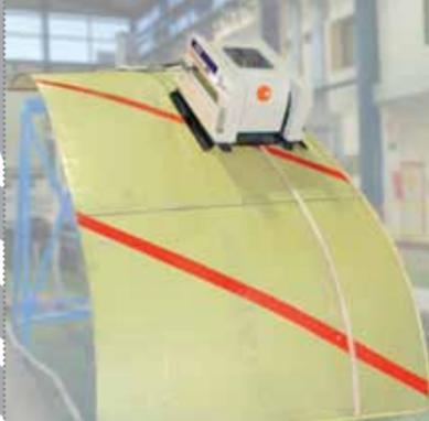
The FDH is a 5 interpolated axis drilling machine with modular design for easy system customization. Its principle is to 'walk' over the aircraft fuselage, holding on place by means of a set of vacuum cups. Once the FDH walks to position, gets locked with the vacuum cups and is ready to perform the drilling/riveting operation.
