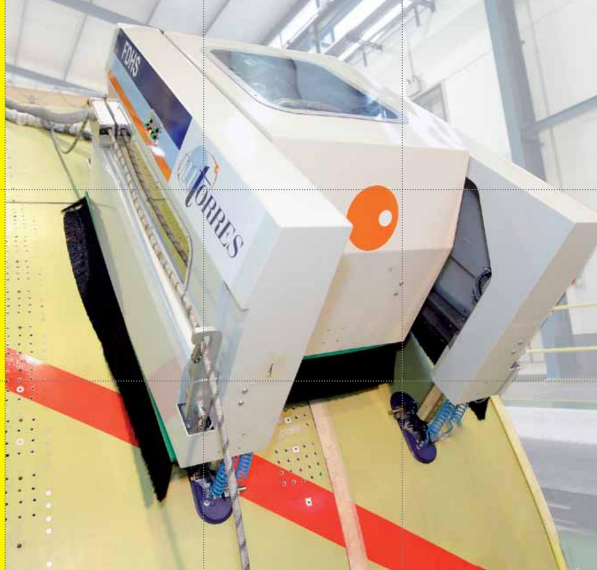
**FLEXIBLE DRILLING HEAD (FDH) 5 Axis Drilling Crawler Robot is a portable and autonomous drilling and riveting stand alone robot.**
