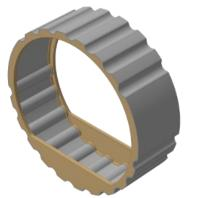
With these solutions, the final structure can integrate frames and omega-shaped stringers without the need of a single rivet.
