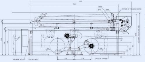
By integrating the <u>TensionFlex</u> into the festoon, we are able to provide accurate tension control, while reducing floorspace. The system is designed to absorb the web tension fluctuations generated from roller inertia during the splice sequence. Our equipment provides accurate tension control throughout the unwinding, splicing sequence, and speed variation of the process.
