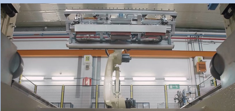
Robot collecting the adhesive tape and attaching it to the preparation arm
