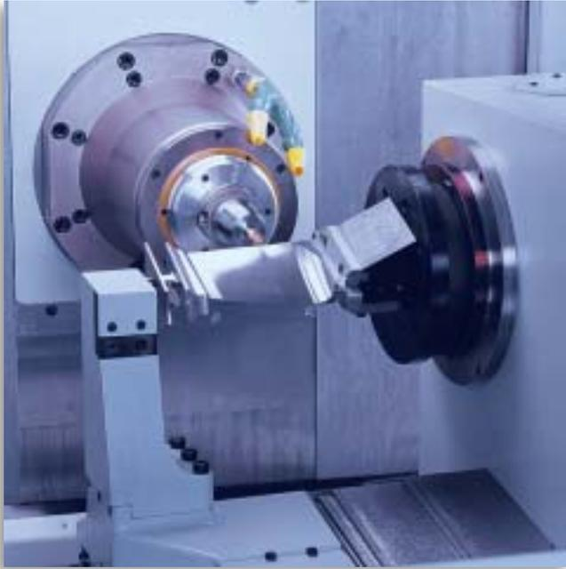
As with most of today's aerospace applications, wall thickness, stepover smoothness, pocket dimensions and floor configurations continue to challenge machining center builders. Typical metal removal is > 90%, in most cases, plus the complex workpieces have webs with extremely thin wall, often unsupported, and thin pocket bottoms.
