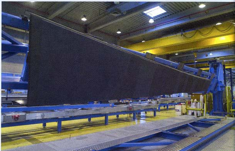
GKN's inner rear spar demonstrator: One of the components that will be produced using MTorres machinery
