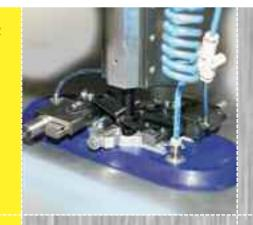
FLEXIBLE DRILLING HEAD (FDH) 5 Axis Drilling Crawler Robot is a portable and autonomous drilling and riveting stand alone robot.
