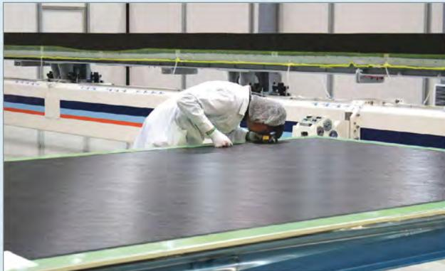
**2** An AeroComposit technician inspects the fiber-placed wingskin, looking for laps, gaps, wrinkles and foreign object debris in the layup. In the background is the tool used to lay up the spar.
