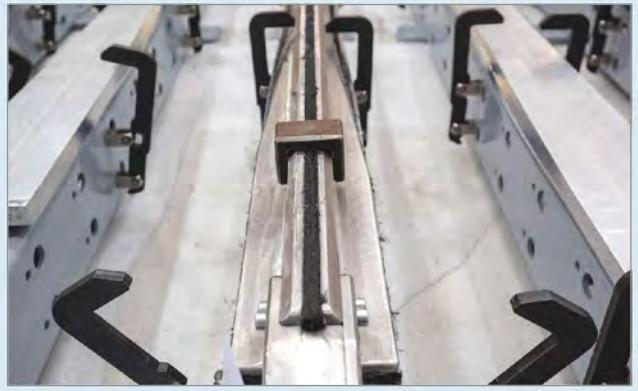
**3** The MS-21 wing stringers are laid up flat and then press-formed into an L shape. Two L-shaped preforms are placed in the tools pictured here, back-to-back, to create the T-shaped stringers that will be co-infused on the upper and lower wingskins.
