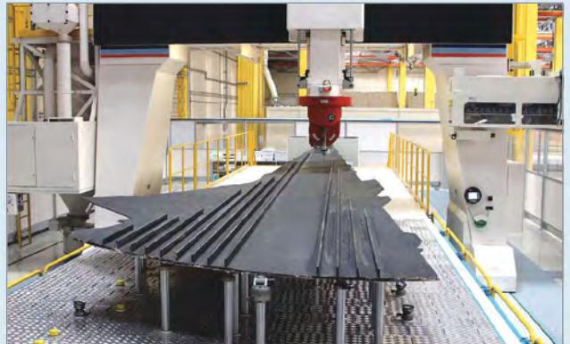
**4** Skins and stringers are vacuum bagged, infused with Solvay's PRISM PE2400 one-part epoxy resin, and cured in a standard oven in a process that takes 8-10 hours to complete. The resulting wingskin with co-infused stringers (shown here) undergoes CNC machining operations — trimming, routing, drilling, cutting — in an MTorres gantry-based system.
