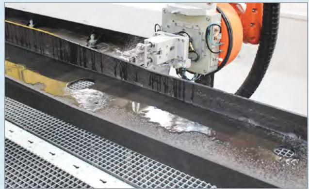
**7** A cured spar undergoes ultrasonic nondestructive inspection. After inspection, the front and rear spar, the metallic ribs and the skins/stringers are assembled with mechanical fasteners.
