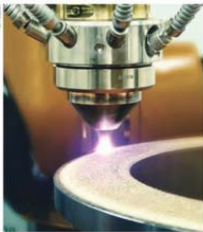
Surface enhancement via direct metal deposition
