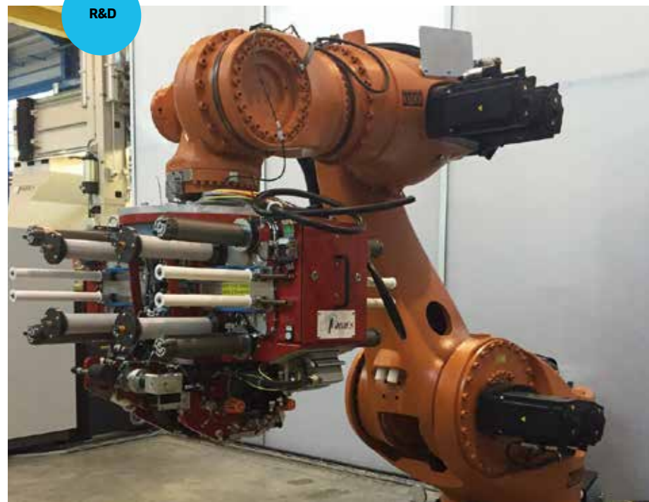
The aim is to create a new AFP platform in a robot for 2D and 3D lamination processes.
