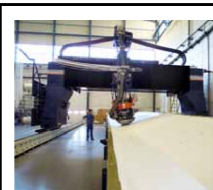
M.Torres past experience on Automatically Lay up of dry glass fiber for Wind Mill blades turned out to be crucial for a fast demonstration of process concept feasibility.
